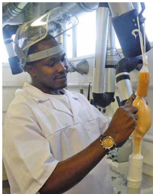
Nkwanga Brian Senabulya learning how to make a prosthesis socket using lamination
