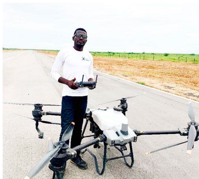
Femi standing with a 40L capacity agricultural spray drone engaged for aerial applications of crop protection and agro-input solutions.
