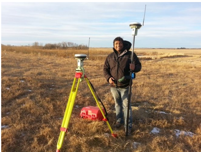
Completing an RTK-GPS survey of field sites for a Digital Elevation Model (DEM).
