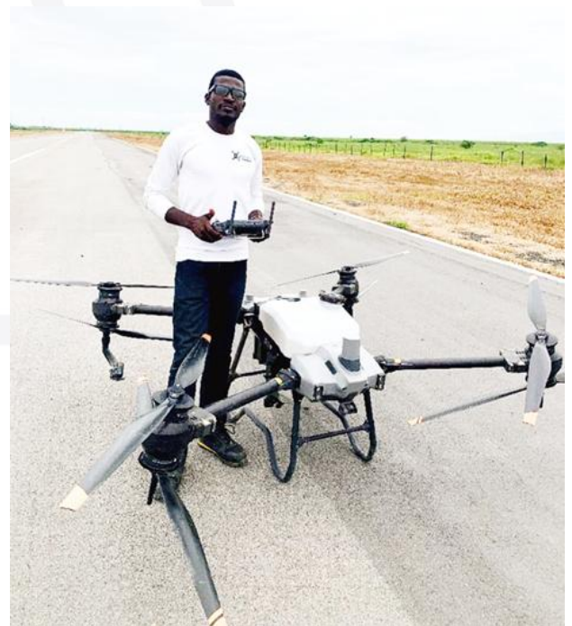
Femi standing with a 40L capacity agricultural spray drone engaged for aerial applications of crop protection and agro-input solutions.
